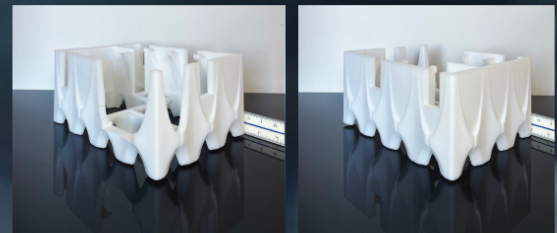
Photographs of 3d print test in ABS material, ensuring geometry is printable without support material.
